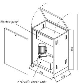
Hydraulic Cabinet, to be sited within 12 metres of the lift shaft. A 100mm conduit run for cables & hoses needs to be provided.
