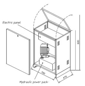
Hydraulic Cabinet, to be sited within 12 metres of the lift shaft. A 100mm conduit run for cables & hoses needs to be provided.
